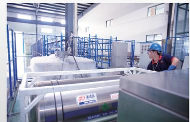
The company has a full set of cryogenic valve test equipment, including full-size liquid nitrogen pool, valve seat leakage flowmeter, torque and test machine, helium detector, to provide capability and product research and development and production test.
