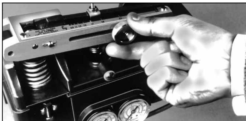
Figure 3: Flow Coefficient Adjustment
