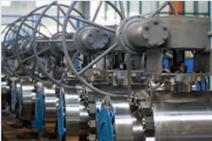
▲ 4" #900 Metal Seated Ball Valves - Full Stainless Steel
